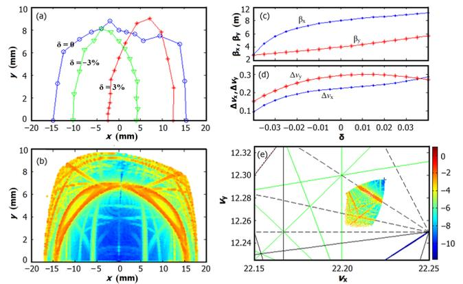
Fig. 3. (Color online) Dynamic aperture, frequency maps, energy detuning of the double-mini- $\beta_y$  optics in the nominal lattice.
