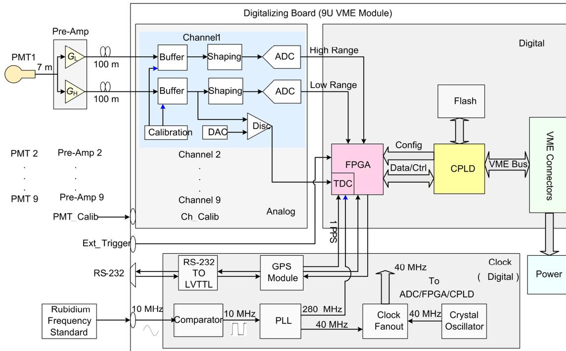
**Fig.1** Architecture of the readout electronics for the prototype WCDA array.
