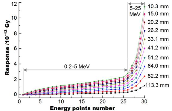
Fig. 3. (Color online) Response of the alanine dosimeters for different energy points and Fe cylinders of different lengths.
