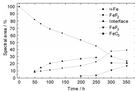
**Fig.3** Spectral areas as functions of milling time for various fractions of  $\alpha$ -Fe/PTFE mixture.
