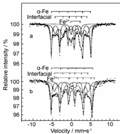
**Fig.2** Mössbauer spectra of the samples Fe/PTFE mixture milled for 140h. (a) Room temperature, (b) 15K.
