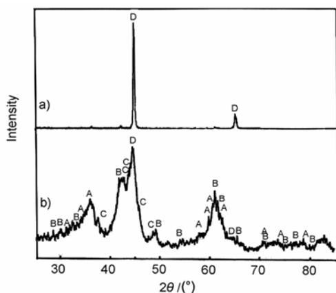
**Fig.4** X-ray diffraction pattern for  $\alpha$ -Fe /PTFE mixture milled for a) 0 h and b) 350 h (A: FeF<sub>2</sub>; B: FeF<sub>3</sub>; C: Fe<sub>3</sub>C; D:  $\alpha$ -Fe ).
