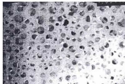
**Fig.5** TEM photograph for the  $\alpha$ -Fe /PTFE mixture milled for 350h.
