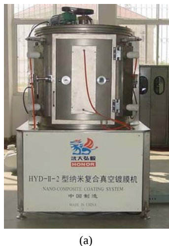
Fig.1 Photograph (a) and schematic cross-section view (b) of the cathode arc enhanced closed-field twin unbalanced magnetron sputter system.
