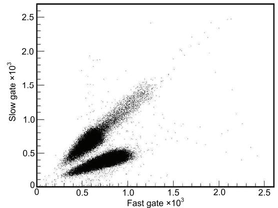
**Fig. 3** The PSD spectrum for CsI(Tl) crystal checked with  $\gamma$  and  $\alpha$  sources, presented in upper and lower bands, respectively. The charge accumulated during the slow gate is plotted against that accumulated during the fast gate.
