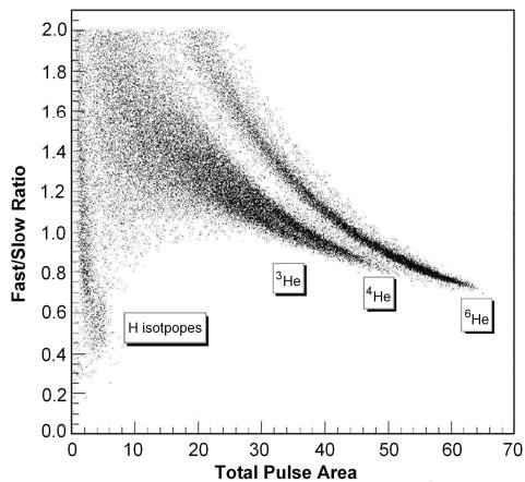
**Fig. 5** Ratio of fast and slow components vs total pulse area.
