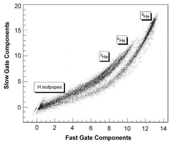
**Fig. 4** Plot of slow gate component versus fast gate component, showing the discrimination of particles.
