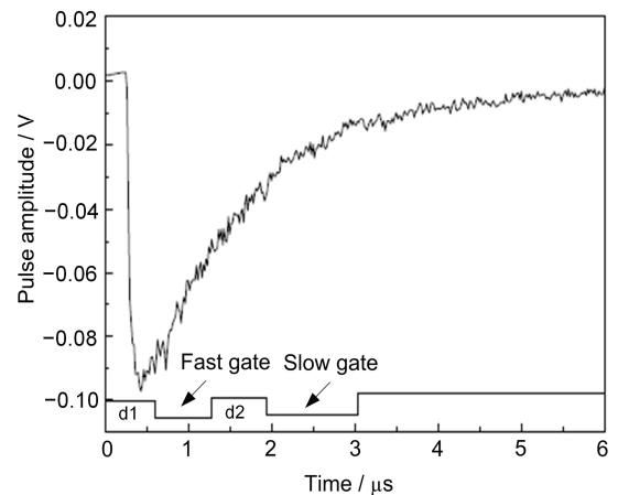
**Fig. 2** One signal of light output from CsI(Tl) crystal.
