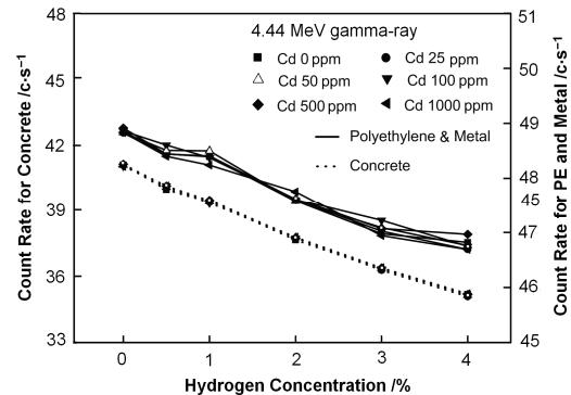
**Fig. 4** Count rate of the prompt  $\gamma$ -ray at 4.44 MeV calculated by MCNP5 with fast neutron activation of carbon (graphite cell), as function of the H and Cd contents in the two materials.
