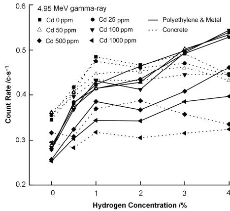
**Fig. 5** Count rate of the prompt  $\gamma$ -ray at 4.95 MeV calculated by MCNP5 with thermal neutron activation of carbon(graphite cell) as a function of the H and Cd contents in the two materials.
