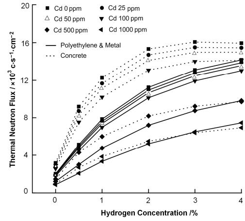
**Fig. 7** Average thermal neutron flux calculated by MCNP-5 varied as function of the hydrogen and cadmium concentration for the two materials.
