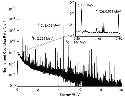
**Fig. 2** Simulated prompt gamma spectrum of concrete sample (115 kg) of 500 ppm cadmium. The simulation was performed by MCNP5 with  $10^8 \text{n}\cdot\text{s}^{-1}$  of 14 MeV neutrons, which was normalized to 1.
