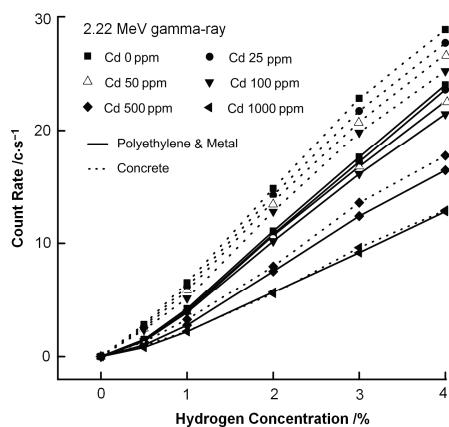
**Fig. 3** Count rate of the prompt  $\gamma$ -ray at 2.22 MeV calculated by MCNP5 with thermal neutron activation of H in the sample, as function of the H and Cd concentration in the two materials.
