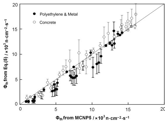
**Fig.8** Comparison of the average thermal neutron flux calculated by mean of Eq.(5) by MCNP5 for the two materials.
