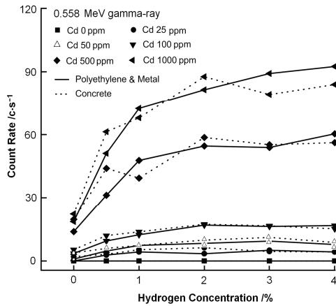
**Fig. 6** Count rate of the prompt  $\gamma$ -ray at 0.558 MeV calculated by MCNP5 with thermal neutron activation of cadmium in the sample as a function of the H and Cd concentration in the two materials.
