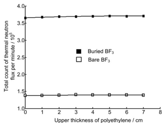
**Fig.5** Comparison between the two configurations, with buried and bare  $\text{BF}_3$  detectors.
