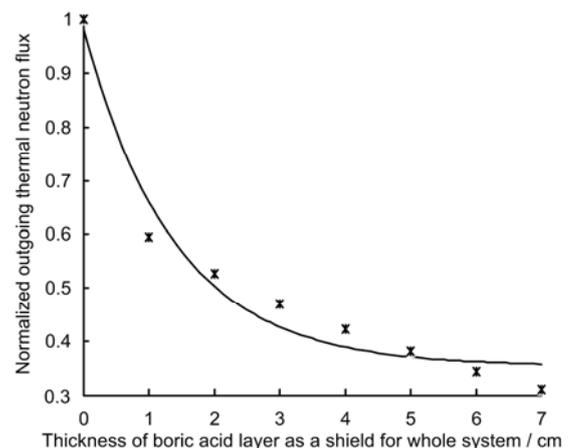
**Fig.3** Outgoing thermal neutron flux vs. the thickness of the boric acid layer when the radius of the cylindrical polyethylene fixed 17 cm.
