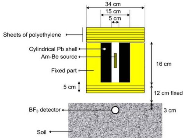
**Fig.1** The land mine detection system details.
