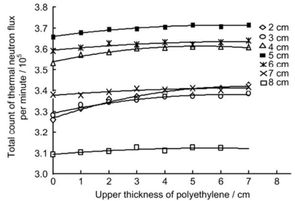
**Fig.4** Total neutron flux per minute using polyethylene at both upper and lower parts.
