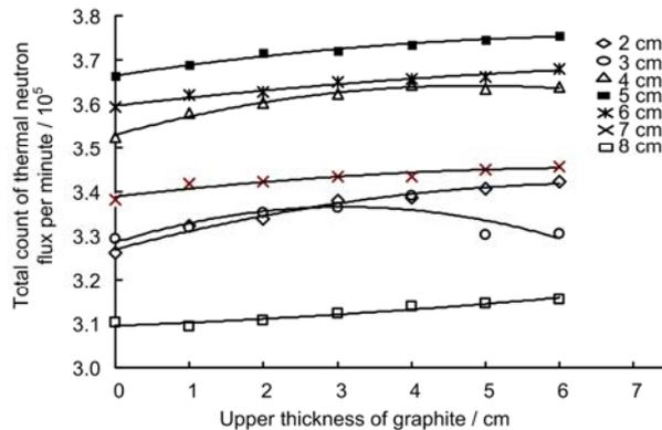
**Fig.6** Total neutron flux per minute using polyethylene for lower and graphite for upper part of assembly.
