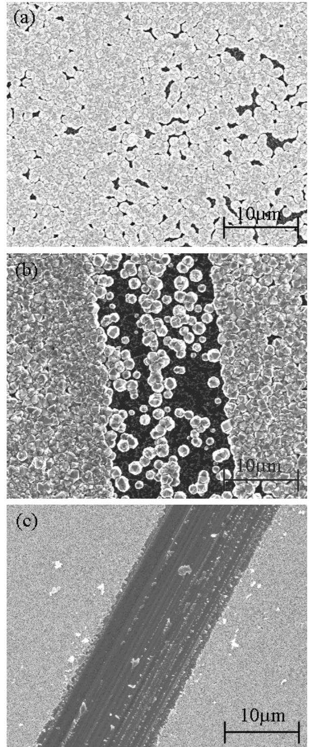
**Fig.3** SEM images of diamond films deposited on silicon wafer scratched by diamond powder (a), the deposited diamond films with needle-scraped pattern on silicon wafer scratched by diamond powder (b) and carbon film scraped by the needle (c).
