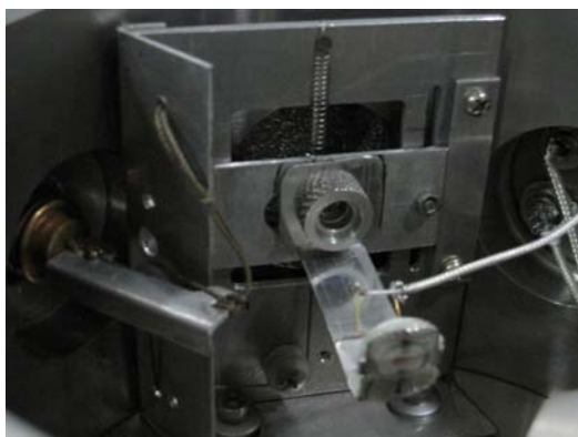
Fig.2 The device that holds the detector.
