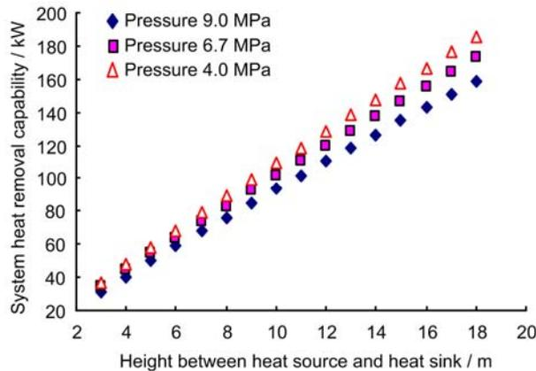
**Fig.7** Residual heat removal capability vs. height between heat source and heat sink.
