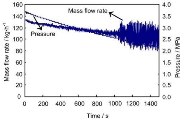
**Fig.6** Typical test of the threshold of height between heat source and heat sink
