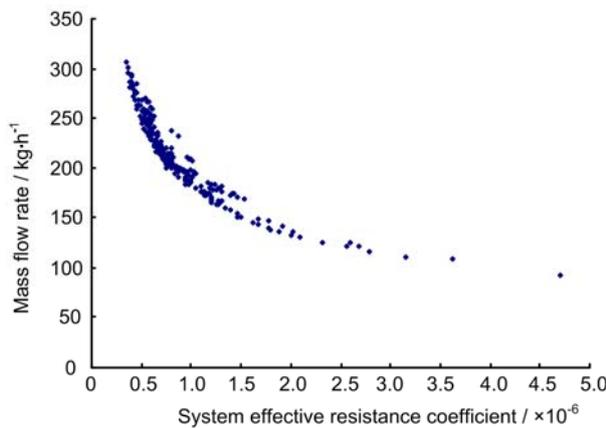
**Fig.10** Mass flowrate of natural circulation vs. system effective resistance coefficient.
