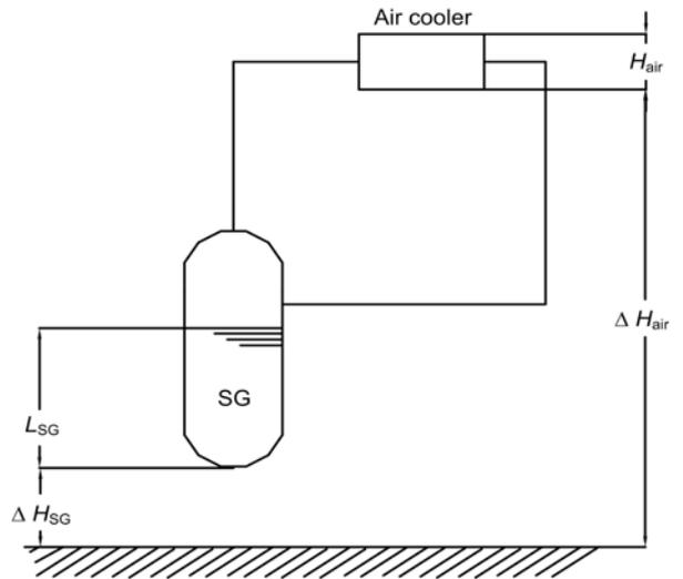
**Fig. 2** Schematic diagram of height between heat source and heat sink.
