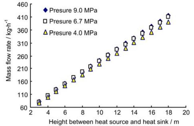
**Fig.8** Mass flowrate of natural circulation vs. height between heat source and heat sink.
