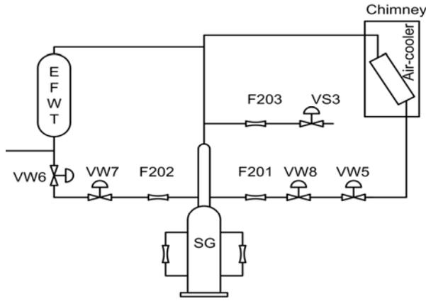
**Fig. 1** Schematic diagram of PRHRS test facility for Chinese advanced PWR.
