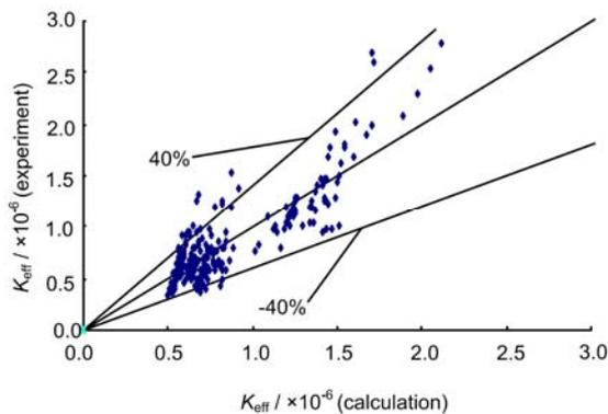
**Fig.4** Experimental and calculated system effective resistance coefficient.
