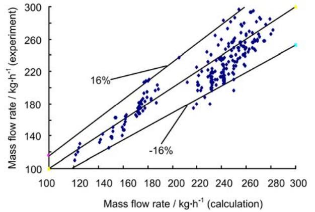
**Fig.5** Experimental and calculated mass flowrate of two-phase natural circulation.
