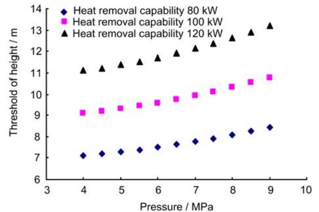
**Fig.9** Residual heat removal capability vs. the threshold of height between heat resource and heat sink.
