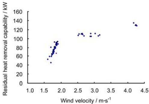
**Fig.11** Residual heat removal capability vs. wind velocity.
