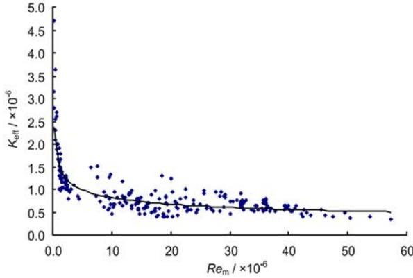
**Fig.3** System effective resistance coefficient vs. modified Reynolds number.
