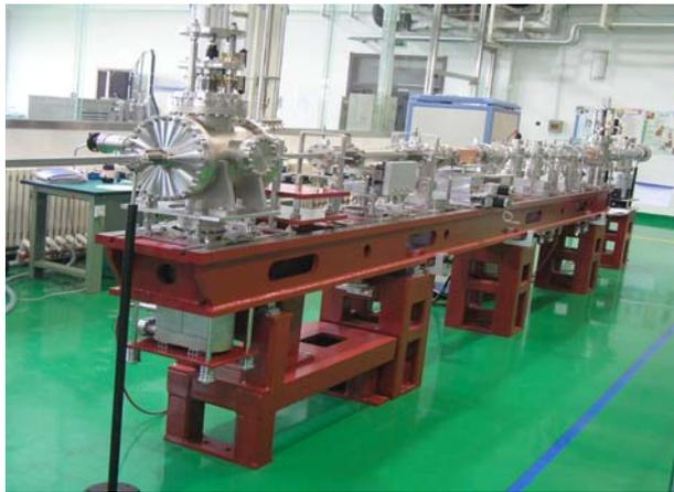
**Fig.8** Pre-installation of a front-end for an undulator beamline
