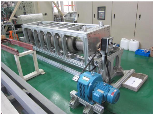
Fig. 1. (Color online) Barrel polishing apparatus for the 500 MHz 5-cell niobium cavity.
