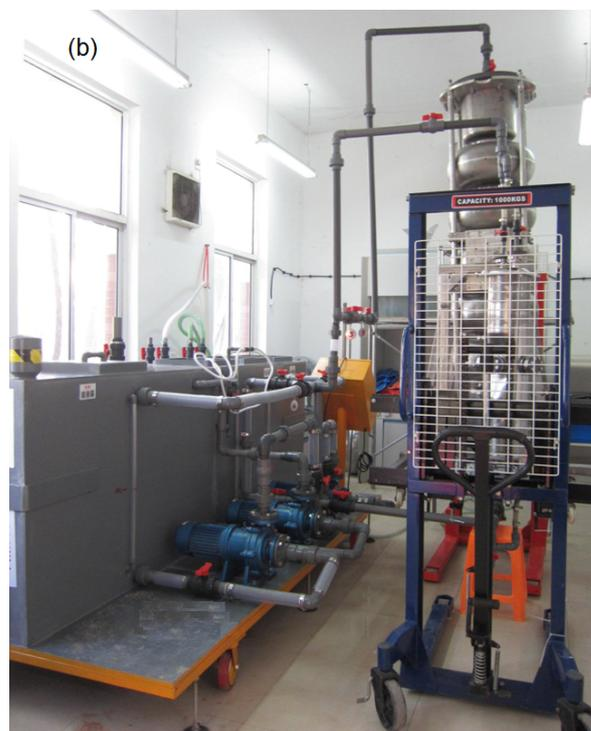
Fig. 2. (Color online) Layout of chemical etching system (a) and apparatus (b) for the two cavities.
