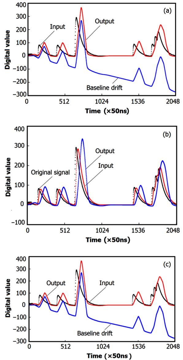
Fig. 6. (Color online) Pulses shaping with (a) the first input data being 0, (b) digital S-K filter processing and (c) the improved recursive algorithm.
