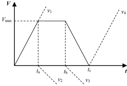
Fig. 1. Synthesis of trapezoidal pulse.
