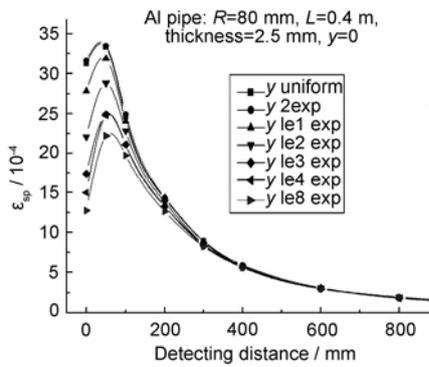
Fig. 5 The  $\varepsilon_{\text{sp}}(d)$  curves of Al pipe.
