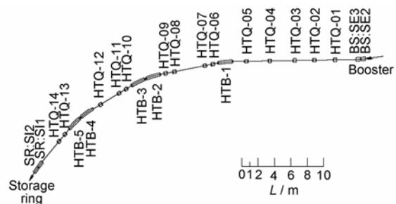
Fig.3 The magnet lattice of HT.
