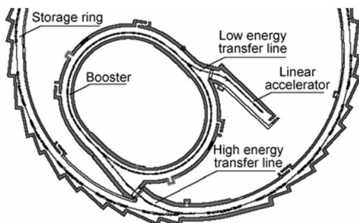
**Fig.1** Schematic layout of the injector.
