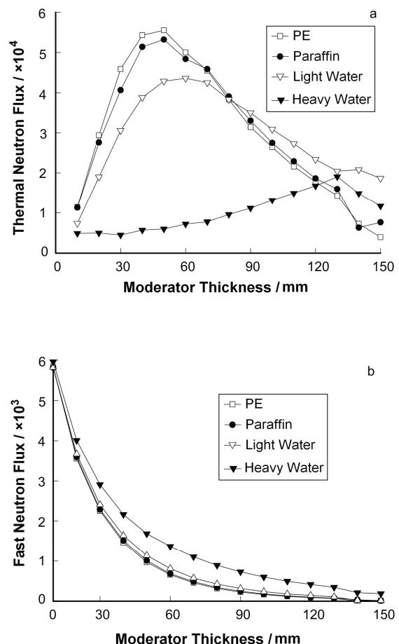
**Fig.3** Thermal (a) and fast (b) neutron fluxes as a function of thickness of different moderator materials.
