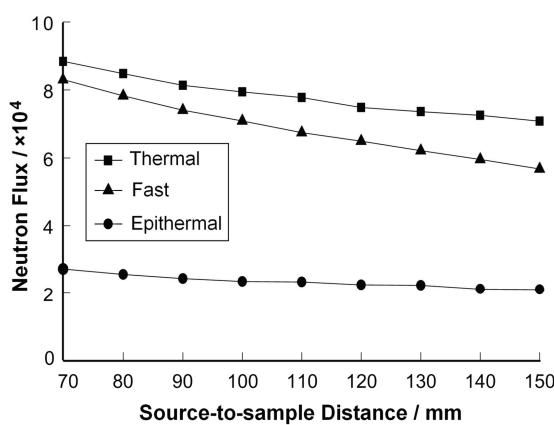
**Fig.4** Flux of thermal, epithermal and fast neutrons, as a function of the source-to-sample distance.
