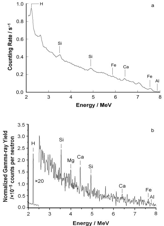
**Fig.8** The measured (a) and simulated (b) spectra of prompt  $\gamma$ -rays from a cement sample.
