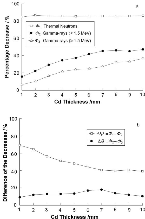
**Fig.6** Percentage decrease of the thermal neutron and  $\gamma$ -ray flux and difference of the decreases vs thickness of Cd sheet.
