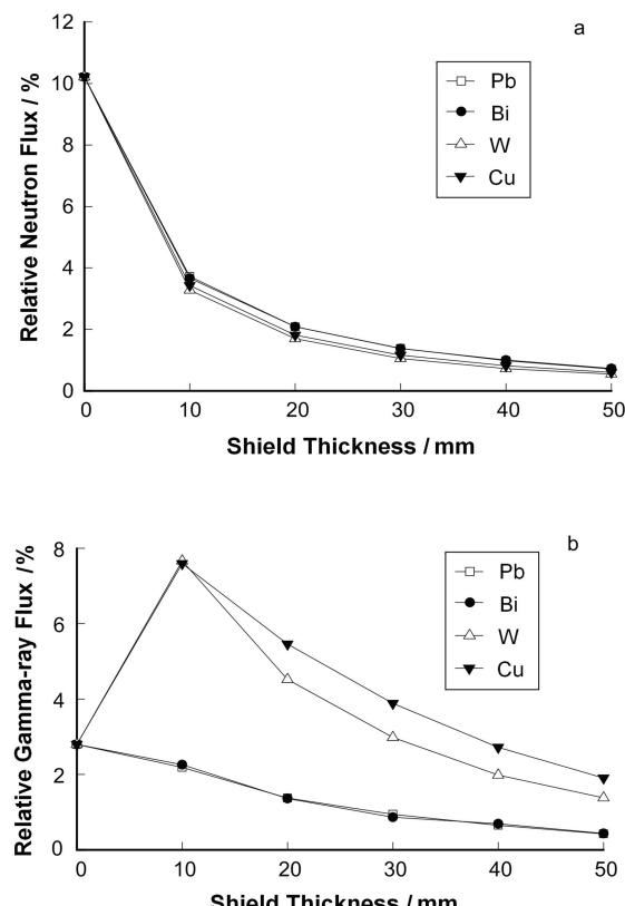
**Fig. 2** Simulated neutron (a) and  $\gamma$ -ray (b) fluxes as function of thickness of different shield materials.
