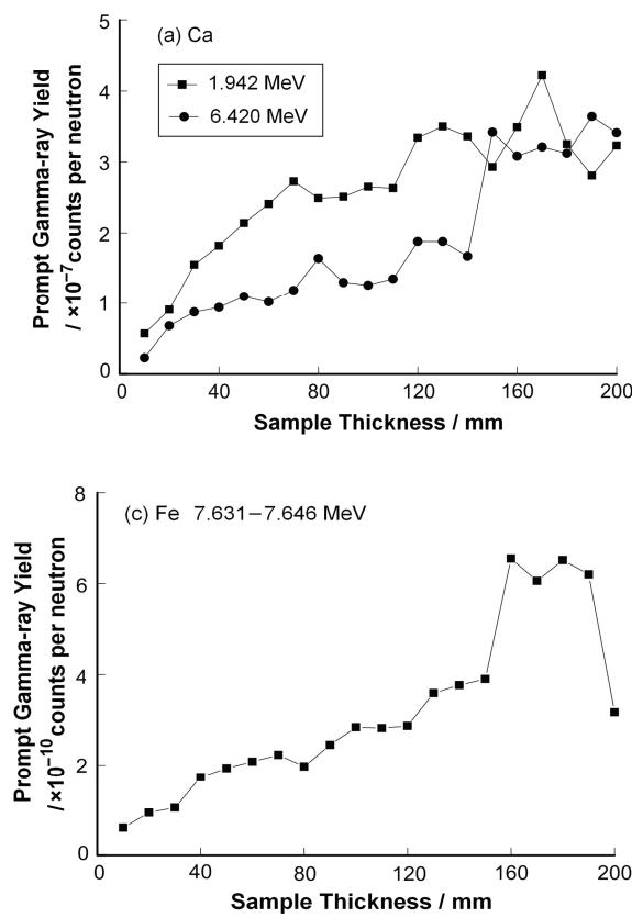
**Fig.5** Normalized yields of prompt  $\gamma$ -rays calculated with elemental targets of different thicknesses.
