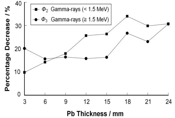
**Fig.7** Gamma-ray yield decrease vs thickness of Pb sheet.
