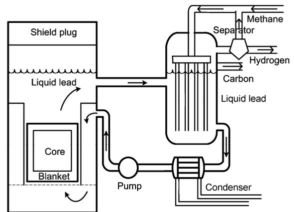
Fig.1 Schematic of a nuclear hydrogen transition system.
