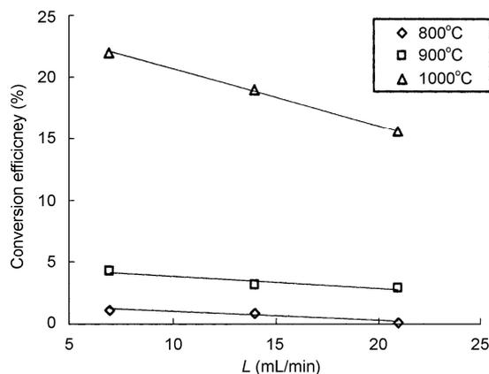
**Fig.4** Conversion efficiency of methane as a function of flow rate.
