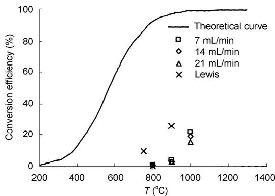
Fig.3 Conversion efficiency of methane as a function of temperature.
