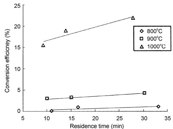
**Fig.5** Conversion efficiency of methane as a function of resident time.
