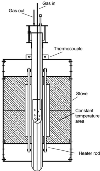
Fig.2 Scheme of pyrolysis reactor.
