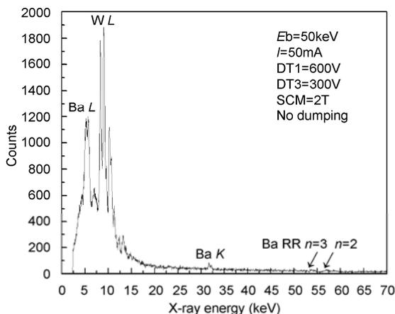
**Fig.2** X-ray spectrum of barium and tungsten ions taken at 50 mA electron-beam current and 50 keV beam energy.
