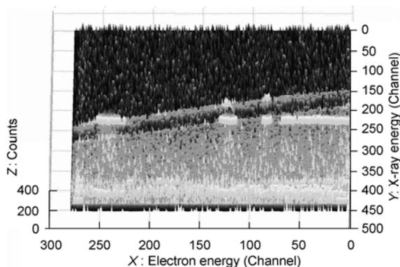
**Fig.3** Di-electronic recombination spectrum for the *KLL* resonances of krypton.
