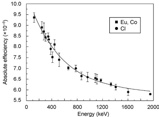
**Fig.4** Absolute efficiency curve up to 2 MeV.
