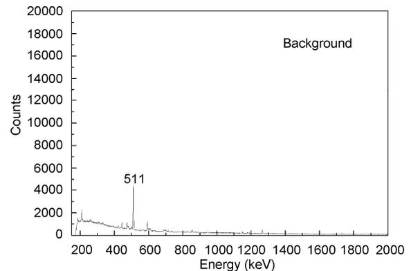
**Fig.3** Background spectrum during reactor operation at full power of 10 MW.
