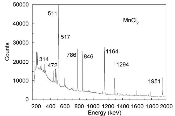
**Fig.1** Prompt gamma ray energy spectrum of  $\text{MnCl}_2$ .
