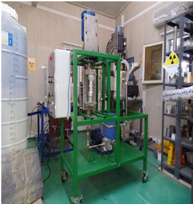
**Fig. 2** (Color online) The TPFHL test-facility. A homogenized two-phase mixture is used to measure the component fraction with a gamma-ray densitometer
