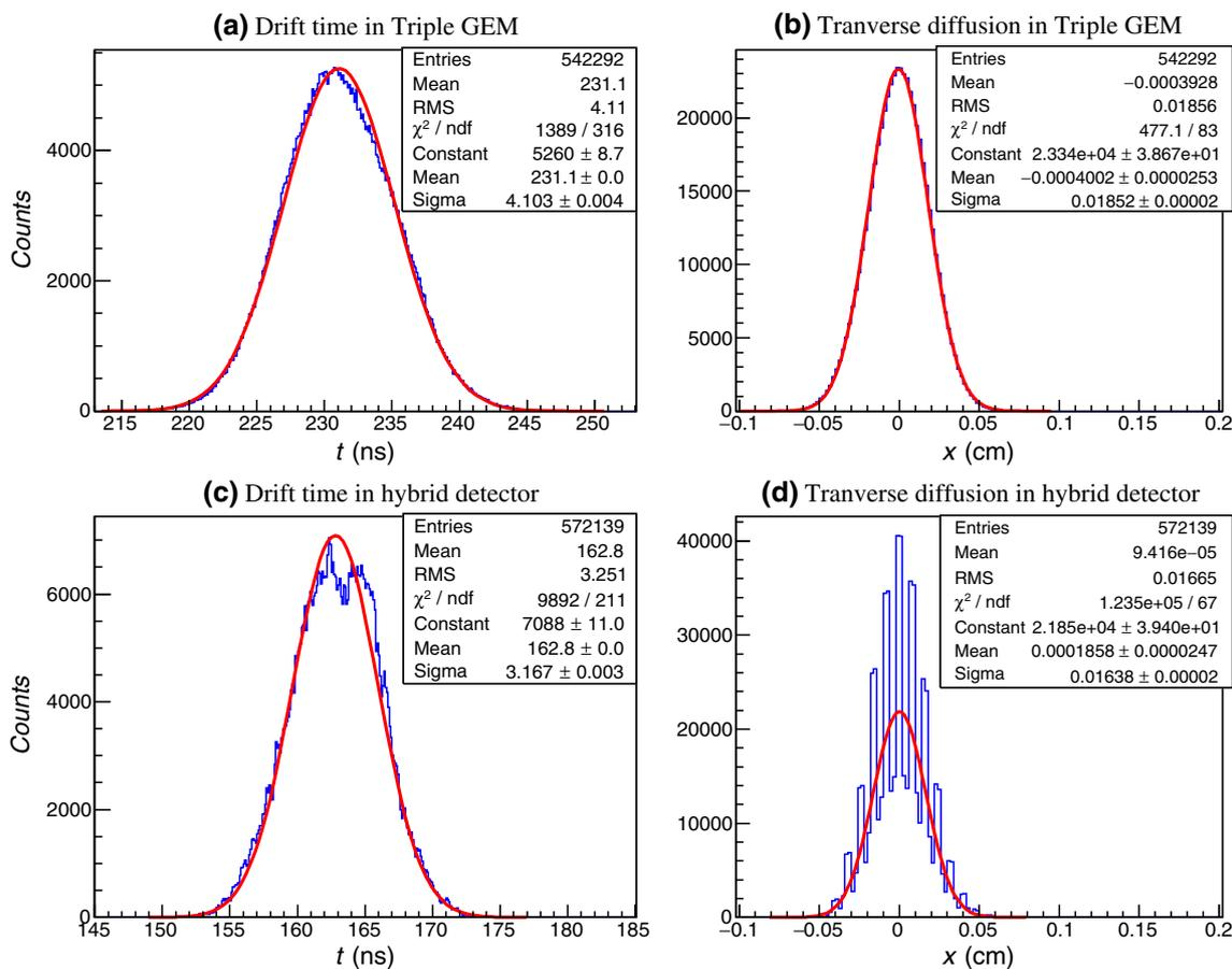
**Fig. 8** Drift time and transverse diffusion of electrons in Triple GEM detector and hybrid detector. The  $t$  axis of drift time represents the time when all the electrons reach PCB-readout and the  $x$  axis of
