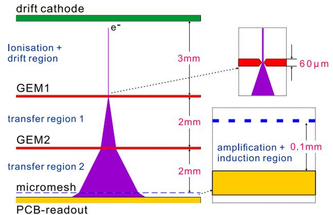
**Fig. 1** (Color online) Structure of the new hybrid detector
