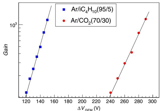
**Fig. 7** (Color online) Gas gain in double GEM for various GEM bias voltages
