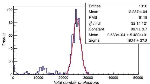
**Fig. 3** (Color online) Energy spectrum of  $^{55}\text{Fe}$  5.9 keV X-ray
