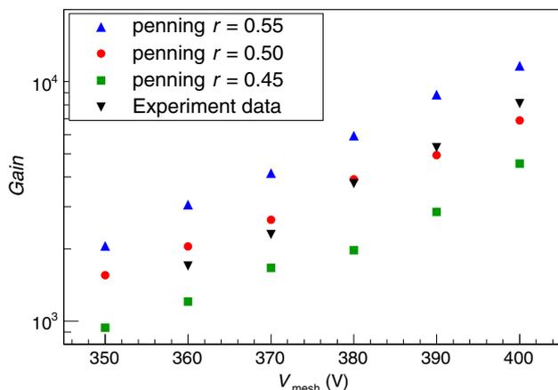
**Fig. 2** (Color online) Penning transfer testing of Micromegas detector. The Exp.Data is from the COMPASS and CLAS12 experiments [4], and it was the biggest gain among the ten different prototypes of Micromegas
