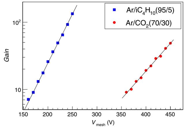
**Fig. 6** (Color online) Gas gain in Micromegas for various mesh voltages
