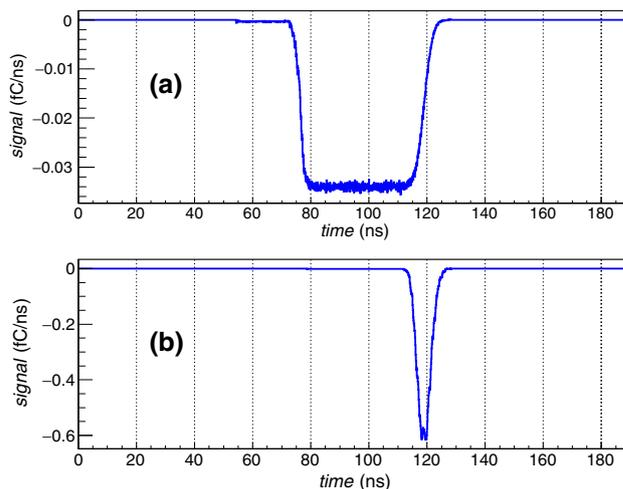
**Fig. 4** (Color online) **a** The current signal of double GEM device; **b** the current signal of hybrid detector. The thickness of the induction region of double GEM device is 2 mm. The working gas mixture of these two devices is Ar/CO<sub>2</sub>(70/30)
