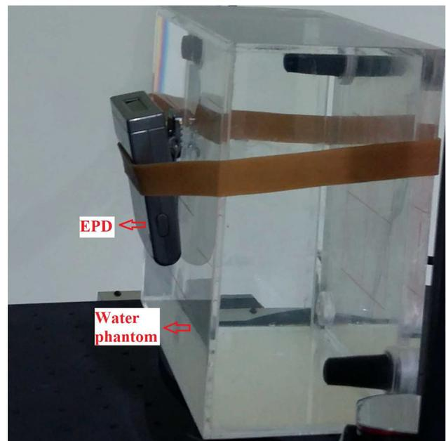
**Fig. 4** (Color online) EPD field measurement setup in the standard laboratory
