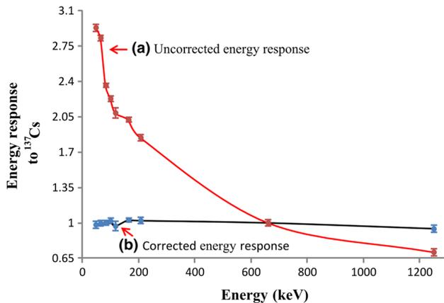
**Fig. 9** (Color online) *a* Uncorrected energy response and *b* corrected energy response
