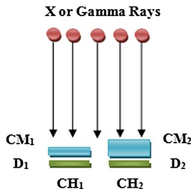
**Fig. 1** (Color online) Schematic of the measurement principle of the two-channel ratio method
