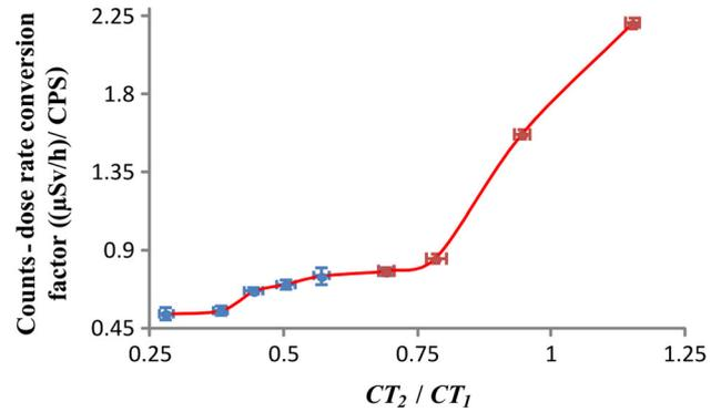
**Fig. 8** (Color online) Counts-dose rate correction factor (CH<sub>1</sub>) as a function of the channel ratio value ( $CT_2/CT_1$ )
