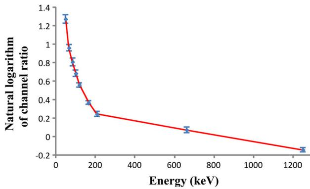
**Fig. 6** (Color online) Natural logarithm of the channel ratio value ( $CT_1/CT_2$ ) as a function of photon energy
