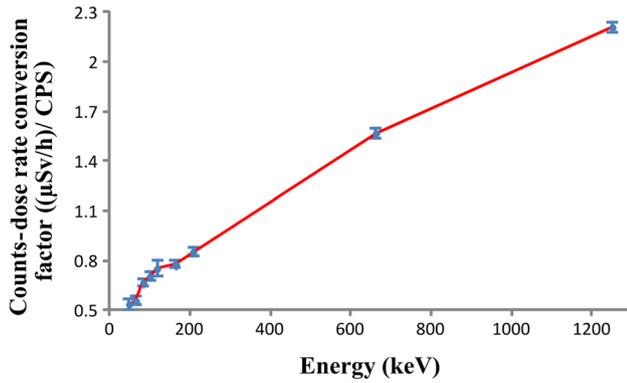
**Fig. 5** (Color online) Counts-dose rate conversion factor of CH<sub>1</sub> as a function of photon energy
