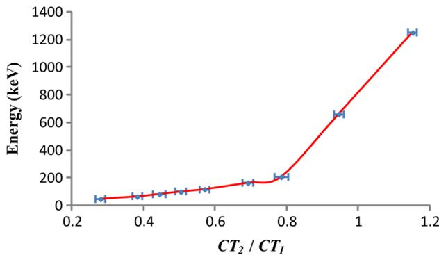
**Fig. 7** (Color online) Photon energy as a function of the channel ratio value ( $CT_2/CT_1$ )
