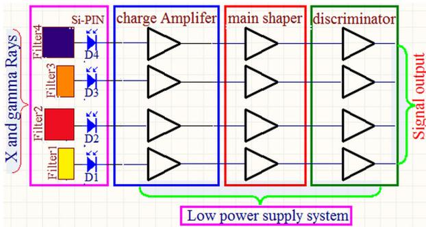
Fig. 2 (Color online) Schematic of the multichannel measurement
