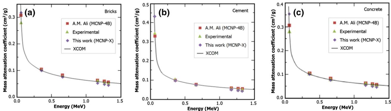
Fig. 2 (Color online) Mass attenuation coefficients of brick (a), cement (b) and concrete (c) samples
