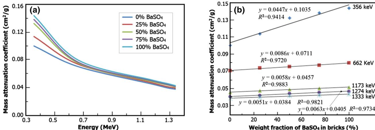
Fig. 3 (Color online) Mass attenuation coefficients of different composites as a function of a energy and b barite weight fraction
