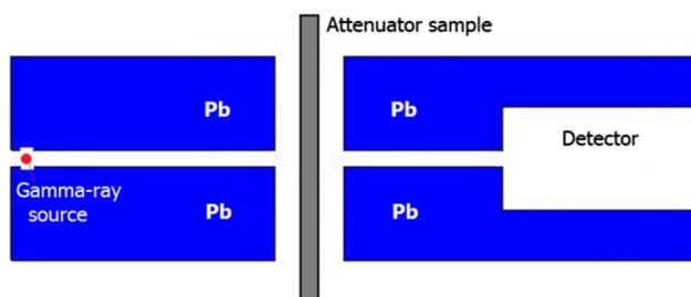
**Fig. 1** (Color online) Schematic view of the MCNP-X simulation geometry
