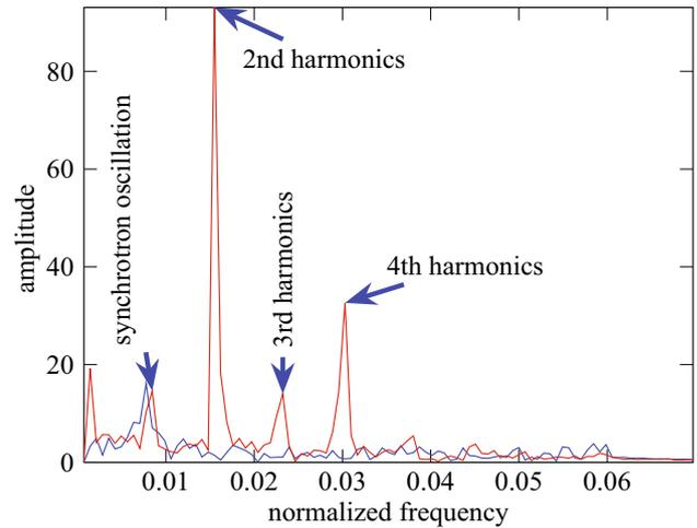
**Fig. 10** (Color online) Spectra of the bunch lengths before and after the injection at the refilled bucket
