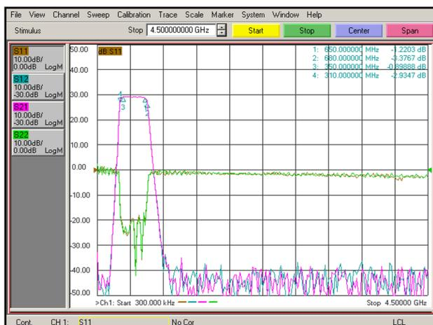
**Fig. 3** (Color online)  $S$ -parameter chart of the 500 MHz filter employed in the measurement system
