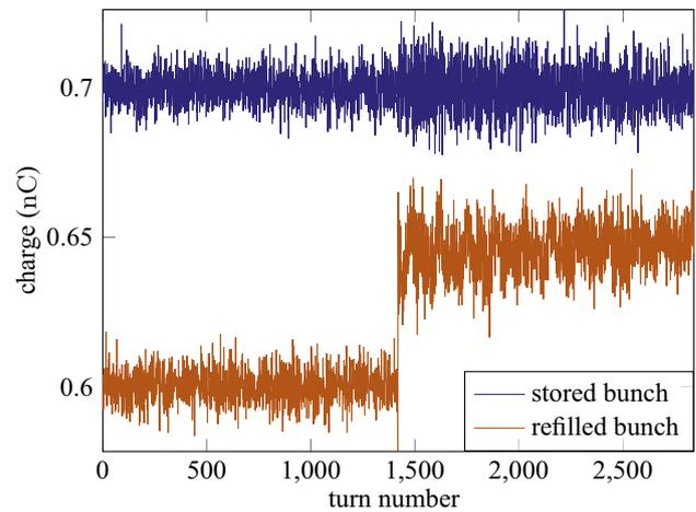
Fig. 6 (Color online) Variation in bunch charge during injecting
