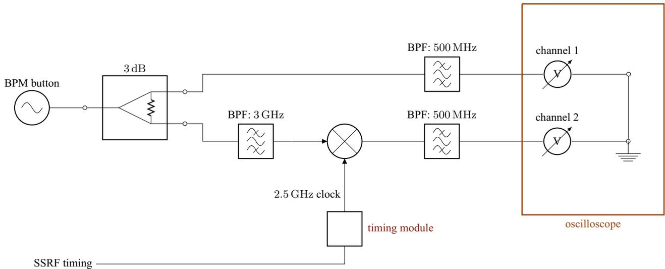
**Fig. 1** (Color online) Block diagram of the bunch length measurement system
