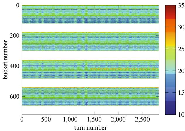
**Fig. 8** (Color online) Waterfall plot of the measured bunch length at each bucket. The injected bunches can be noticed since their lengths oscillate up to 35 ps (the dashed, dark red line around the 400th row)
