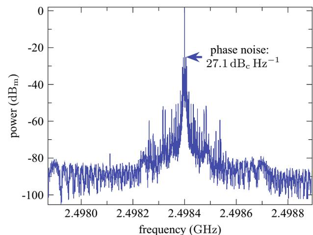
**Fig. 4** (Color online) Amplitude response spectrum of EVAL-ADF4351 programmable wide band frequency synthesizer (ADI Corp.) employed in the measurement system
