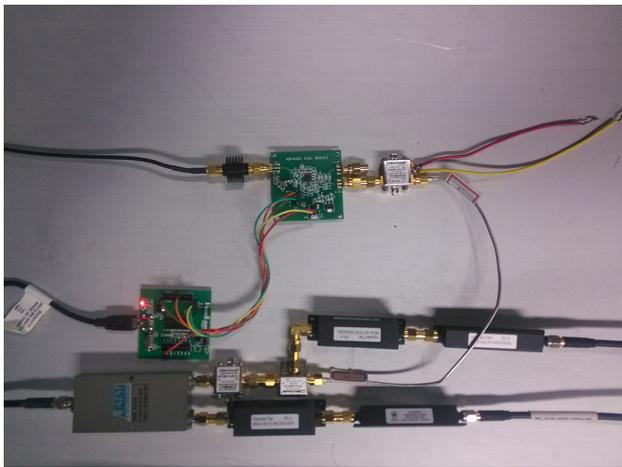
**Fig. 2** (Color online) Photograph of the RF front-end electronics
