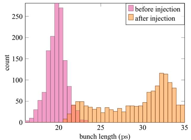
**Fig. 11** (Color online) Histogram of the bunch lengths before and after the injection
