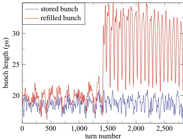
**Fig. 9** (Color online) Synchronous oscillation of bunch length
