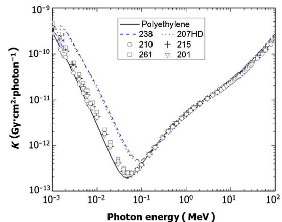
**Fig. 3** Gamma-ray kerma coefficients for neutron shielding materials and polyethylene as a function of photon energy
