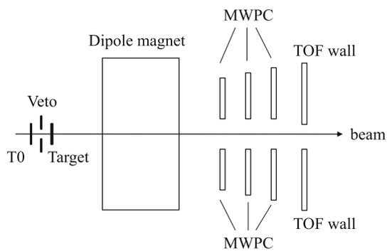
**Fig. 1** Sketch of the top view of the experiment setup at ETF
