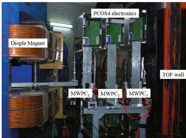
**Fig. 2** (Color online) The experimental setup at ETF. Three MWPCs were assembled and tested at ETF
