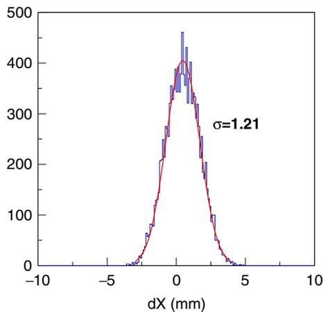
**Fig. 5** (Color online) Deviation between the calculated position and the hit wire in the  $x$  direction
