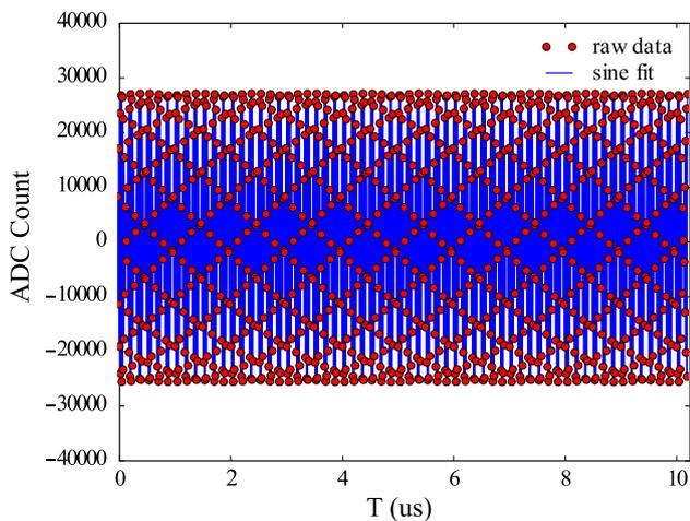
**Fig. 9** 1k points AD9268 ADC1 raw data and sine fit
