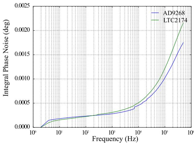
**Fig. 19** The integral differential phase noise for ltc2174/ad9268 boards respectively when measuring 47 MHz signal
