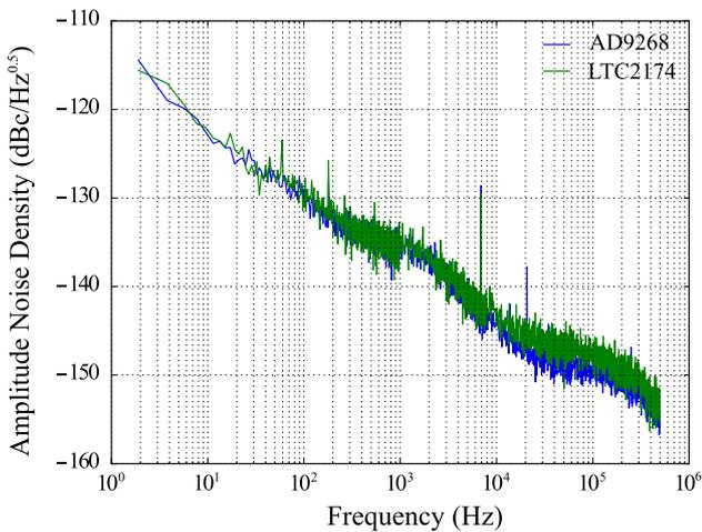
**Fig. 14** The 47 MHz signal amplitude noise density measured by ltc2174/ad9268 boards, respectively
