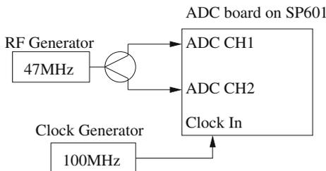
Fig. 7 ADC test setup for additive phase noise and amplitude noise measurement
