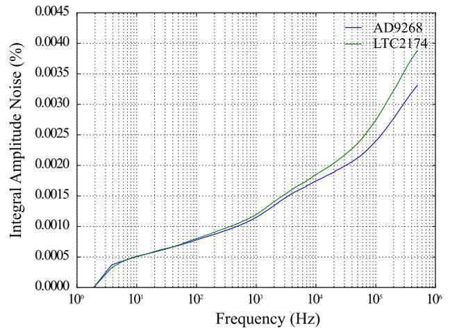
**Fig. 15** Integral amplitude noise of 47 MHz signal measured by ltc2174/ad9268 boards, respectively
