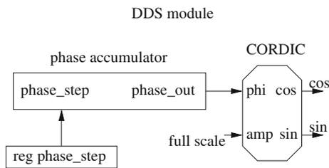
Fig. 6 DDS module structure for LO signal generation
