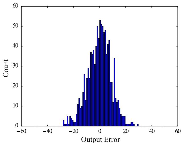
**Fig. 11** 1k points AD9268 ADC1 sine fit error histogram
