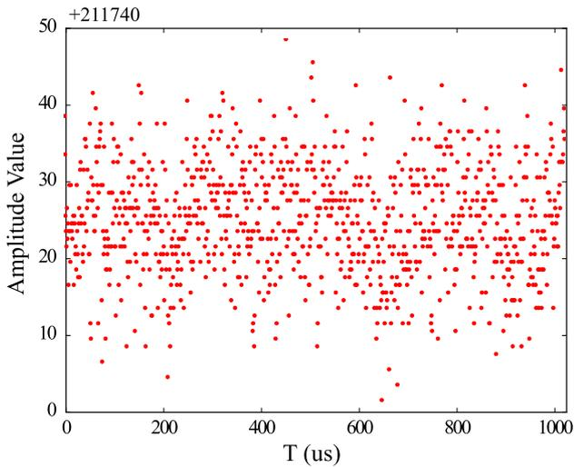
**Fig. 13** The amplitude value of 47 MHz signal measured by ad9268 channel 1
