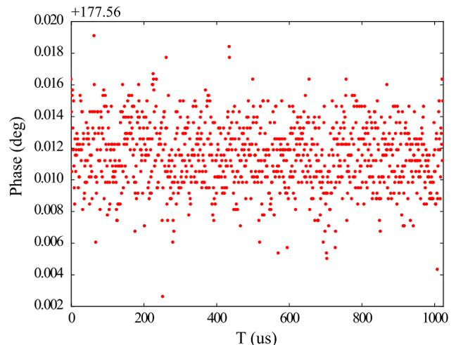
**Fig. 17** The measured phase difference between channel 1 and channel 2 for ad9268 board when measuring 47 MHz signal
