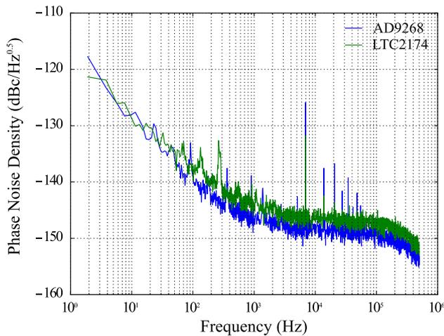
**Fig. 18** The measured differential phase noise density for ltc2174/ad9268 boards respectively when measuring 47 MHz signal
