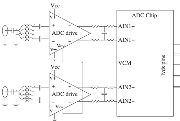
**Fig. 1** ADC test schematic design
