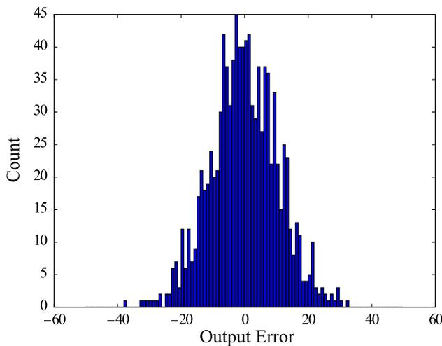
**Fig. 10** 1k points LTC2174 ADC1 sine fit error histogram
