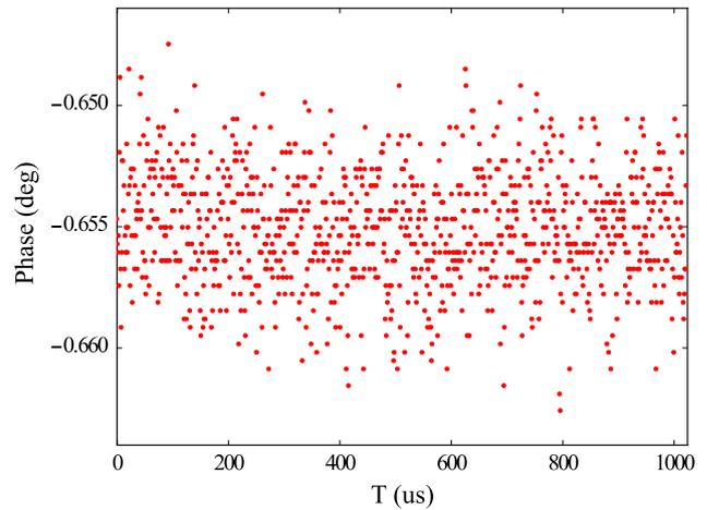
**Fig. 16** The measured phase difference between channel 1 and channel 2 for ltc2174 board when measuring 47 MHz signal
