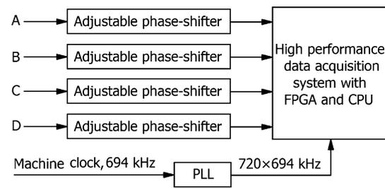
**Fig. 2** Hardware architecture of the bunch-by-bunch beam position measurement system
