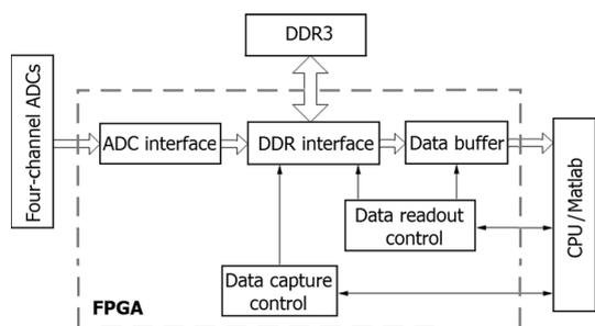
**Fig. 3** Logic design in FPGA
