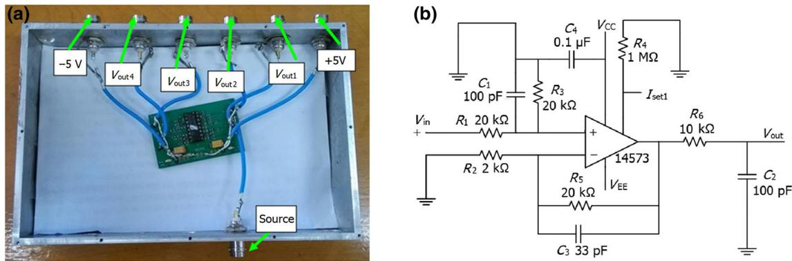
Fig. 9 The experiment set-up (a) and circuit of the op-amp circuit, (b) the schematic diagram of the set-up
