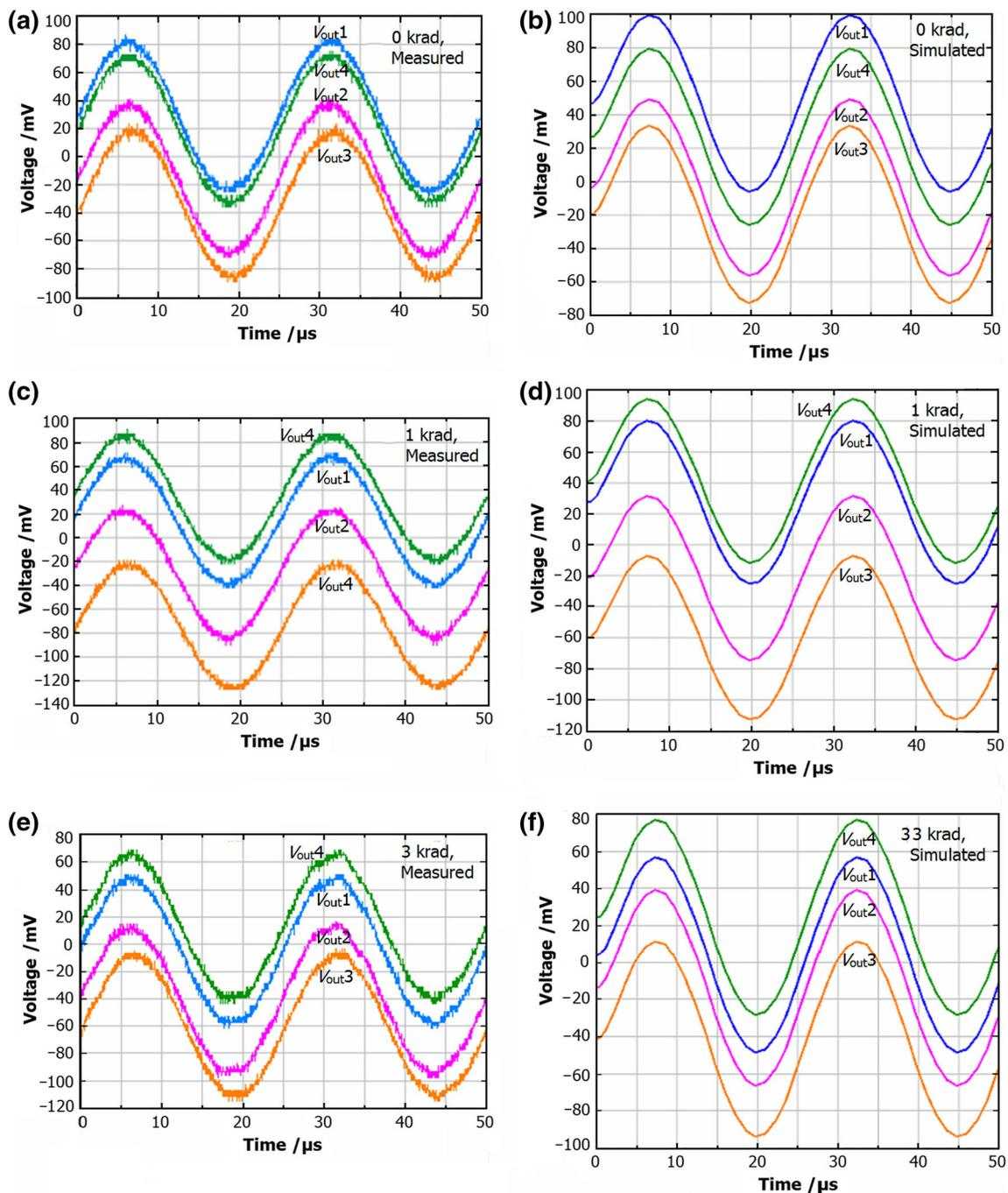
**Fig. 11** Experiment and simulation results at 0–3 krad, with 10 mV sine input
