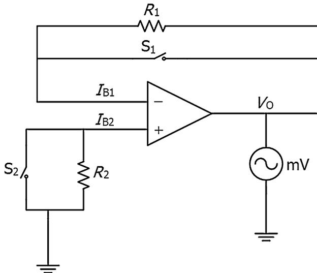
Fig. 3 The test circuit for  $I_B$
