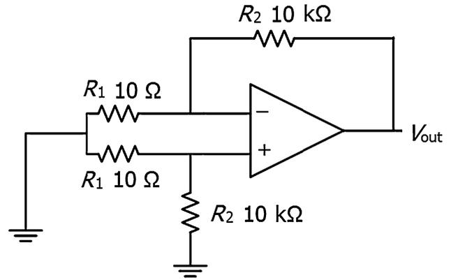
Fig. 4 The test circuit for  $V_{OS}$
