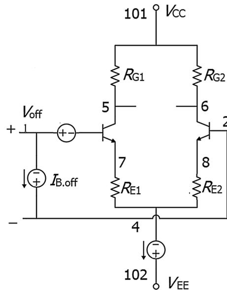
Fig. 2 The input offset voltage and the bias current model
