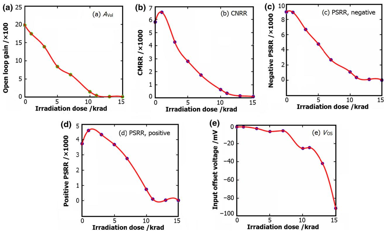
Fig. 10 Parameters of the MC14573 irradiated to different TIDs
