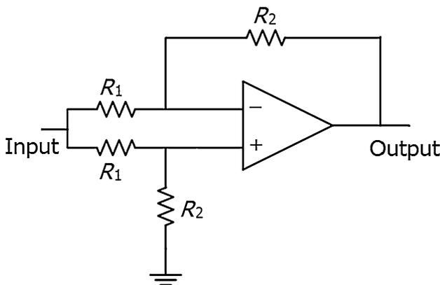
**Fig. 6** The test circuit for CMRR
