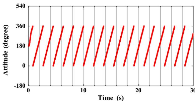
Fig. 8 Yaw of the detector in the rotary test
