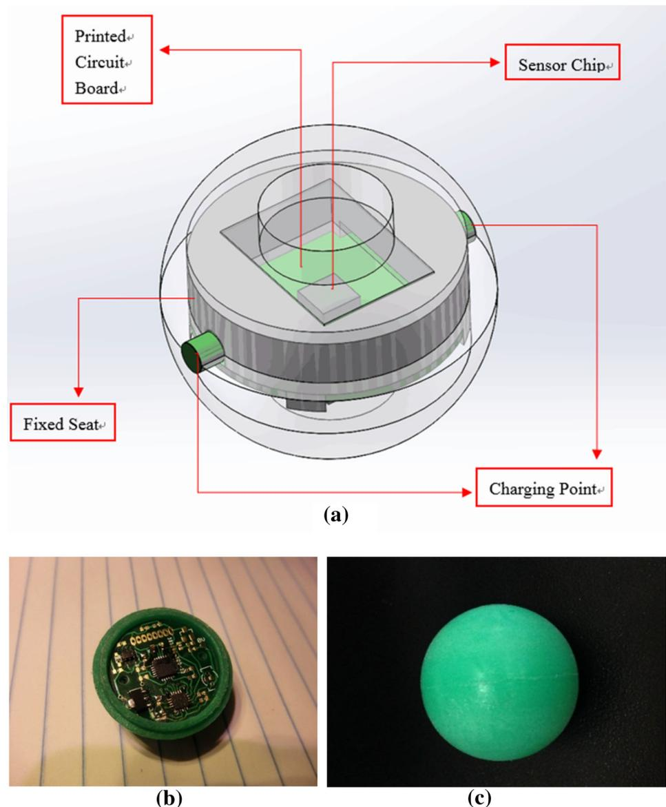
antenna are carefully optimized for better performance in the pebble bed. We use 2.4 GHz and 433 MHz frequencies for different experiments. The detector also contains flash memory, a thermistor and a rechargeable battery, as shown in Fig. 1b, c.
