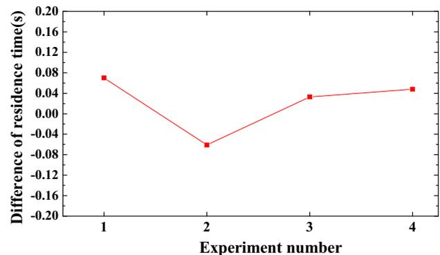
Fig. 12 The difference of the residence times measured by the pebble detectors and the high-speed camera
