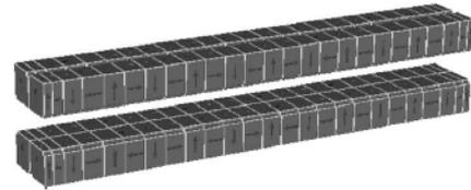
**Fig.2** Four magnet arrays of the undulator.
