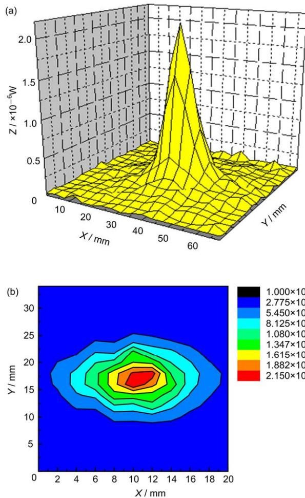
**Fig.5** Surface plot (a) and contour plot (b) of the spatial power distribution 50 mm away from the glass window.
