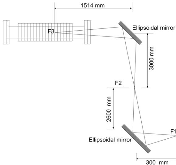
**Fig.3** Sketch of the infrared beam transfer line.
