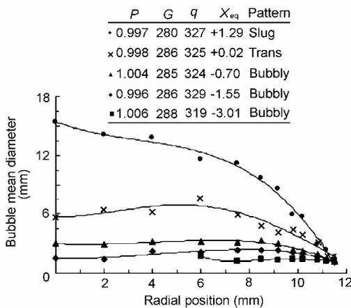
Fig.3 Radial profiles of bubble mean diameter.
