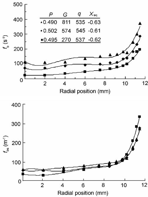
Fig.5 Effect of mass flux on  $f_b$  and  $f_{bs}$  radial profiles.
