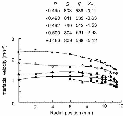
Fig.2 Radial profiles of interfacial velocity.
