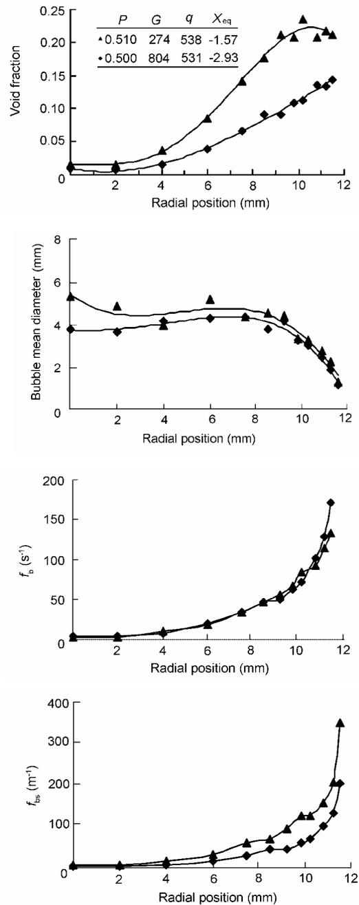
Fig.6 Contrast between  $f_{bs}$  and  $f_b$ .
