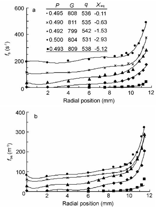
Fig.4 (a) Effect of equilibrium quality on  $f_b$  radial profiles; (b) Effect of equilibrium quality on  $f_{bs}$  radial profiles.
