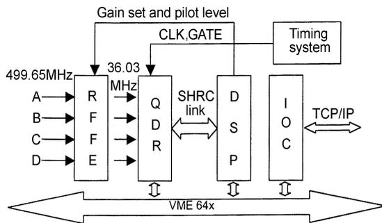
Fig.1 Block diagram of DBPM system.
