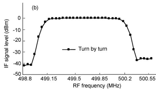
Fig.2 (a) Bandwidth of RF front end module; (b) system bandwidth for turn-by-turn mode.
