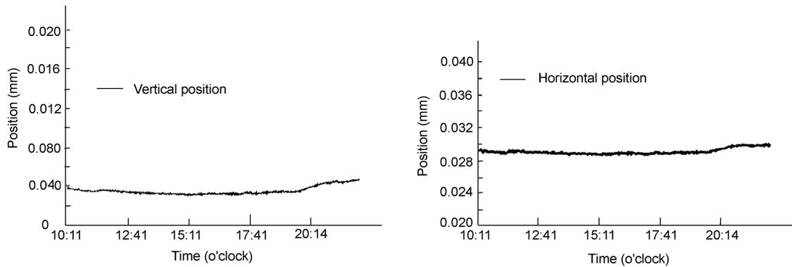
**Fig.5** Long term stability of the SSRF DBPM system. It's within  $\pm 1\mu\text{m}$  over a time period of 12 hours.
