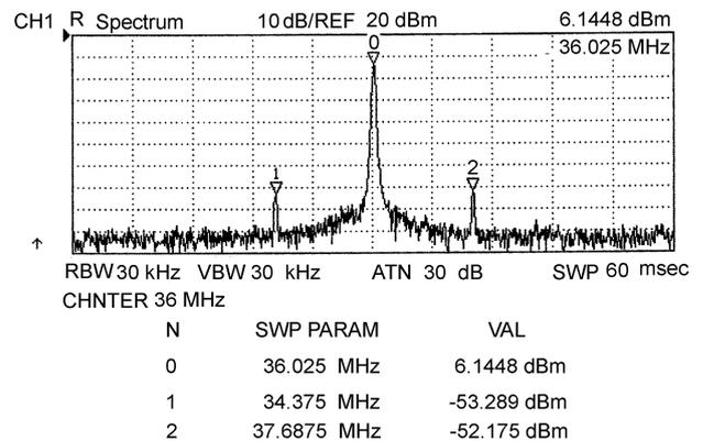
Fig.4 A spectrum of IF signal. Carrier signal @36.025 MHz; pilot signal @34.375 MHz.
