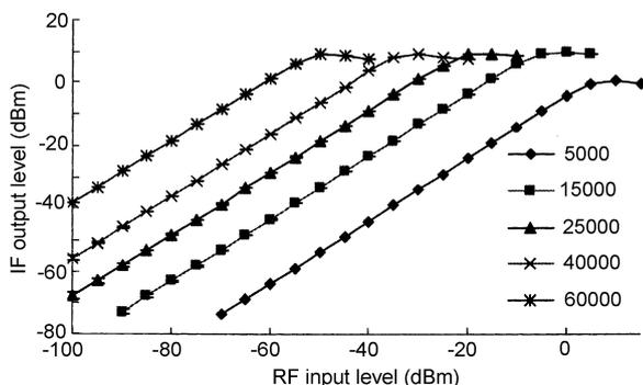
Fig.3 IF amplitude vs. RF amplitude relationship for different gain setting.
