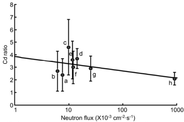
**Fig.4** Dependence of cadmium ratio on flux of thermal and epithermal neutrons (see Table 1).
