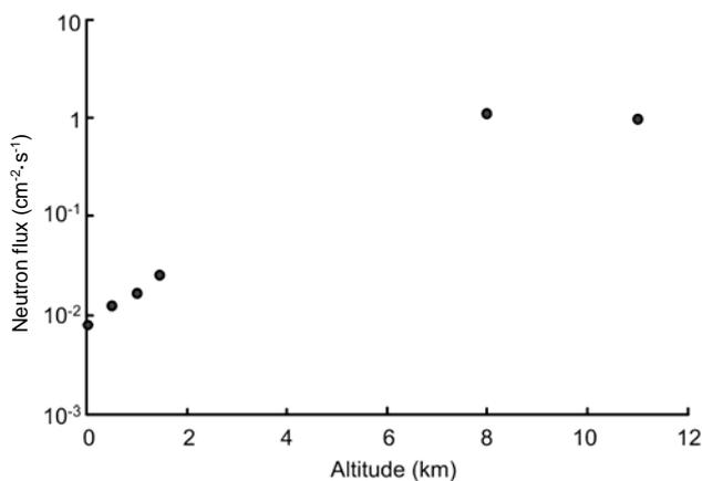
**Fig.1** Variation of slow neutron flux with the altitude.
