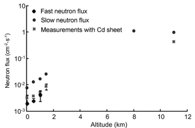
**Fig.2** Variation of average neutron fluxes with the altitude.
