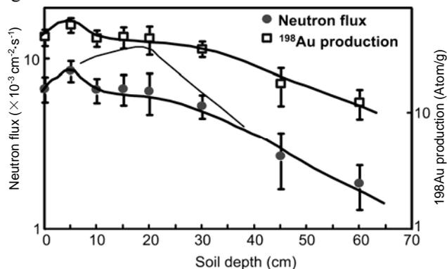
**Fig.6** Variation of thermal neutron flux and  $^{198}\text{Au}$  production with the depth of ground.
