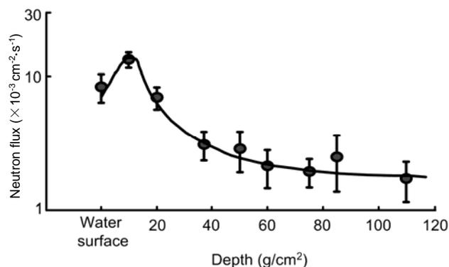
**Fig.5** Thermal environmental neutron flux as a function of depth in fresh water.
