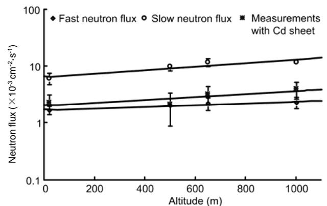
**Fig.3** Variation of neutron fluxes inside concrete buildings with the altitude.
