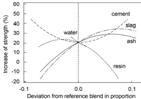
**Fig.3** Trace plot for the increase of strength (reference blend: water 0.18, slag 0.17, ash 0.17, cement 0.26, resin 0.22).
