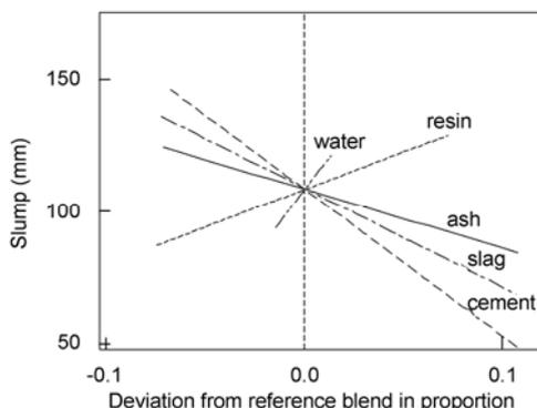
**Fig.6** Trace plot of slump (reference blend: water 0.18, slag 0.17, ash 0.17, cement 0.26).
