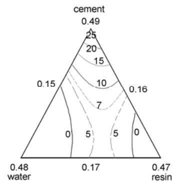
**Fig.2** Contour plot for 28-day strength (MPa) in cement, water and resin (slag=0.10, ash=0.10).
