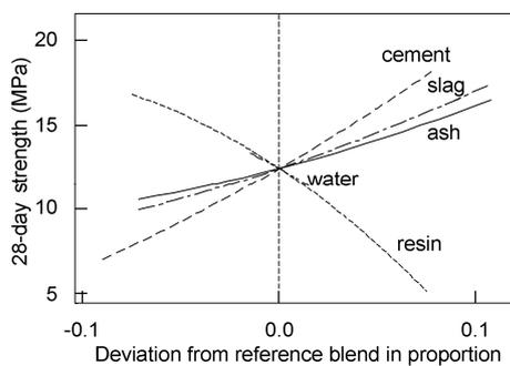
**Fig.1** Trace plot for 28-day strength (reference blend: water 0.18, slag 0.17, ash 0.17, cement 0.26, resin 0.22).
