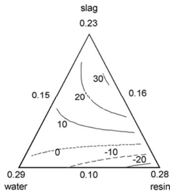
**Fig.4** Contour plot for the increase of strength (%) in slag, water and resin (ash=0.10, cement=0.27).
