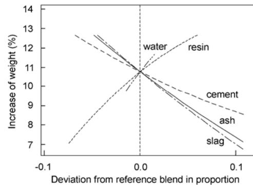
**Fig.5** Trace plot for the increase of weight (reference blend: water 0.18, slag 0.17, ash 0.17, cement 0.20, resin 0.22).
