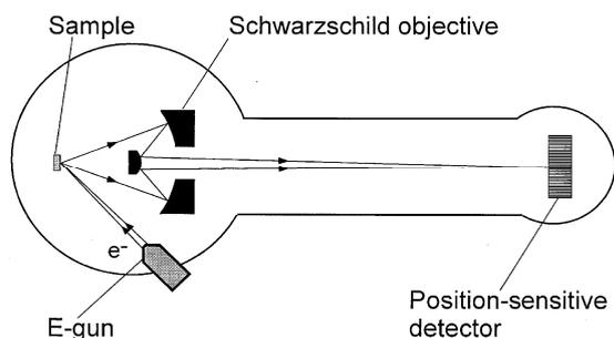
**Fig.8** Schematic of soft X-ray emission imaging microscope.<sup>[23]</sup>
