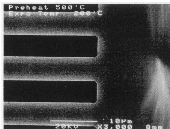
**Fig.10** SEM image of the test sample.<sup>[23]</sup> The dark area is  $\text{SiO}_2$  and the bright area is W, both 5  $\mu\text{m}$  in width.
