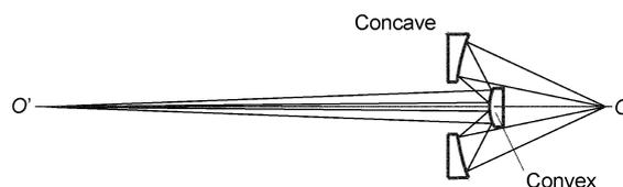
**Fig.1** Schematic of Schwarzschild objective.
