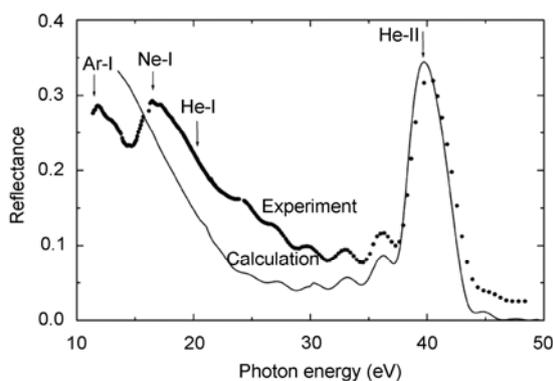
**Fig.6** Reflectance spectrum of SiC-Mg/Y<sub>2</sub>O<sub>3</sub> two-color multilayer.<sup>[15]</sup> Arrows indicate energy positions of not only He- I and He- II, but also Ar- I and Ne- I resonance lines.  $\theta=10^\circ$ .
