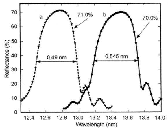
**Fig.4** Reflectance spectra of (a) Mo/Si and (b) Mo/Be multilayers.<sup>[11]</sup> In between Mo and Si, and in between Mo and Be, layers of  $B_4C$  are inserted to prevent diffusion.
