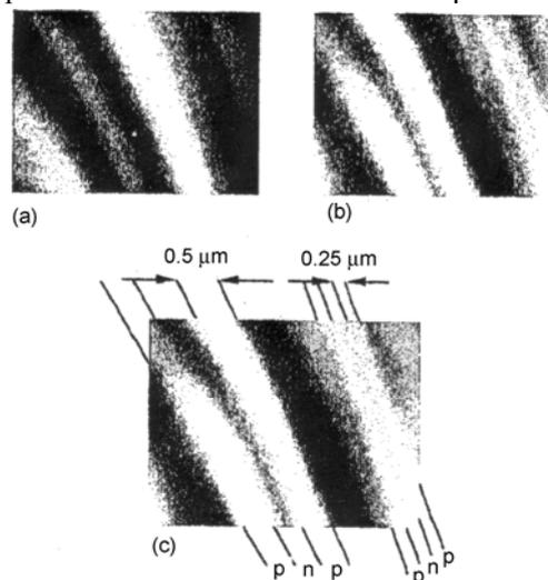
**Fig.7** Cross-sectional image of an MBE-grown p-n GaAs superlattice with different periods obtained by sample scanning.<sup>[22]</sup> The two top images are obtained by tuning the energy analyzer at the kinetic energy of the Ga 3d peak of (a) n-type GaAs and (b) p-type GaAs. The layers of n-type GaAs appear bright in (a) and dark in (b). Image (c) is the difference between the two top images.
