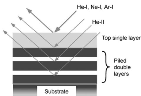
**Fig.5** Structure of two-color multilayer for He- I and He- II resonance lines.<sup>[15]</sup>
