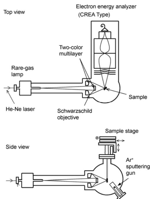
**Fig.12** Schematic of ultraviolet photoelectron scanning microscope.<sup>[25]</sup>
