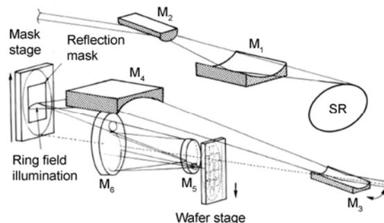
Fig.15 Schematic of demagnifying optics for fabrication of ultra large scale integrated (ULSI) circuits.<sup>[28]</sup> SR means synchrotron radiation source.
