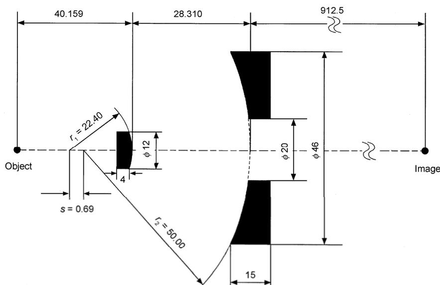
**Fig.9** Schwarzschild objective in eccentric arrangement.<sup>[23]</sup>
