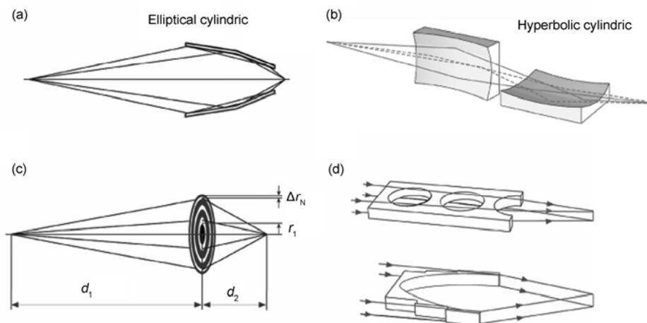
**Fig.2** Schematics of objectives. (a) Wolter type, (b) Kirkpatrick-Baez type, (c) zone plate, (d) refraction lens.
