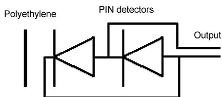
**Fig.1** Structure of the compensation detector.
