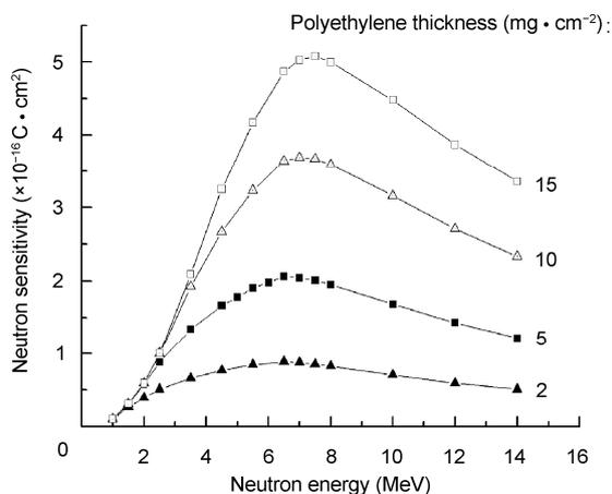
**Fig.3** Response of detector to neutrons with different energies.
