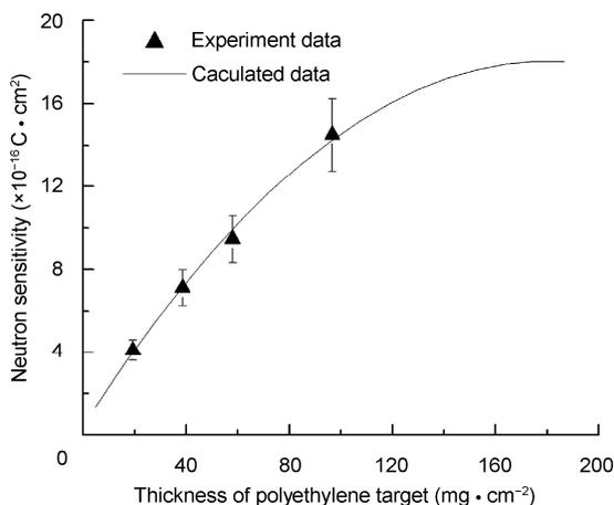
**Fig.2** Relation between sensitivity and thickness of polyethylene target.
