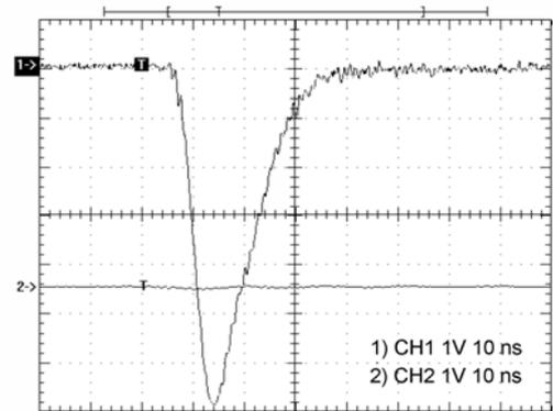
**Fig.5** Output signals from the compensation detector and usual PIN detector ignited by the same impulse  $\gamma$  radiation.
