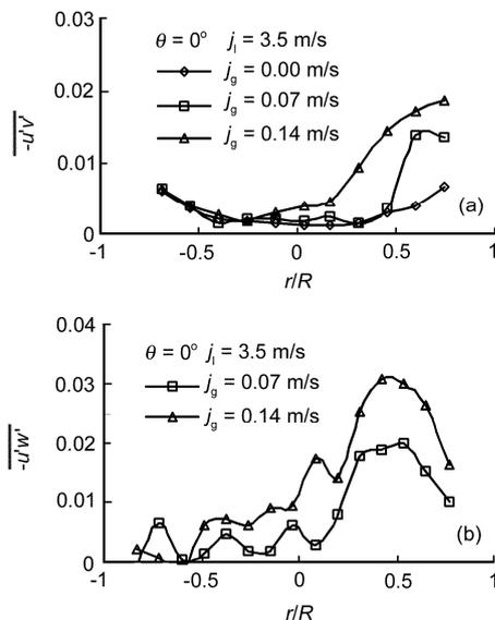
Fig.7 Liquid-phase turbulent stress.
