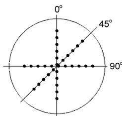
**Fig.2** Probe positions across test section.
