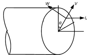
**Fig.3** The cylindrical coordinate system.
