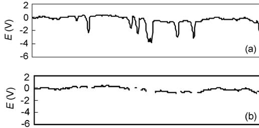
**Fig.4** Raw and filtered hot-film signal. (a) Raw signal; (b) Filtered signal.
