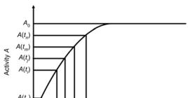
**Fig.1** Change of activity of daughter nuclide with sealing time in a secular radioactive equilibrium system.
