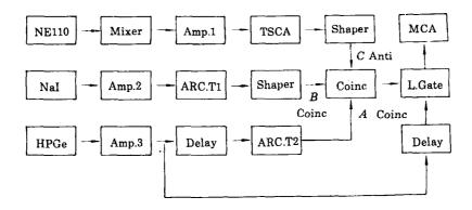
Fig.1 Electronics block diagram of the coincidence—anticoincidence spectrometer with the Compton suppression
