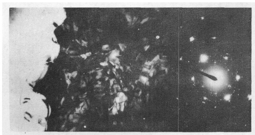
Fig.3 Transmission electron microscope results from sample B ( 1.5 \text{ MeV } 1 \times 10^{16} \text{ Si/cm}^2 at 250^\circ\text{C} )
