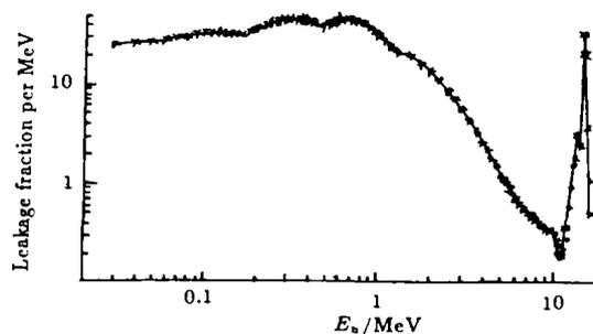
**Fig.1** Leakage spectrum of D-T neutrons from iron shell of 10 cm thickness
