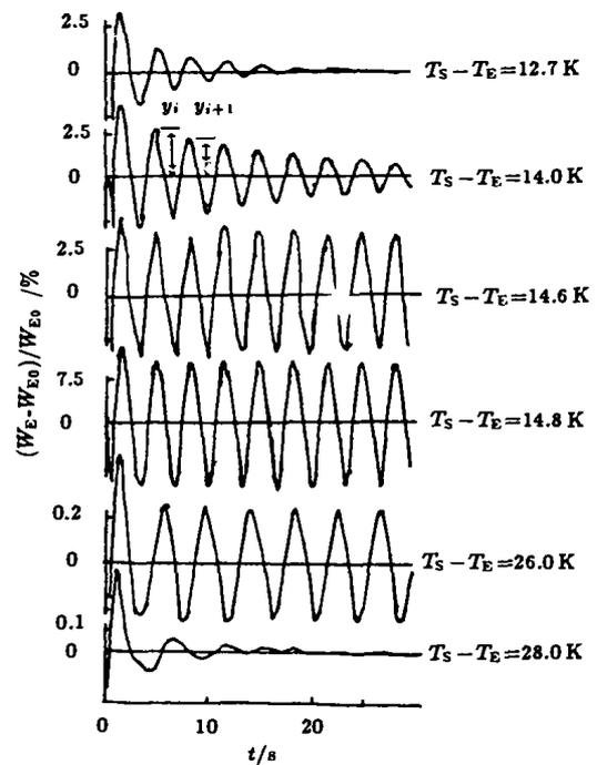
Fig.3 Relative oscillation amplitude of the inlet velocity  $W_E$  for different inlet subcoolings  $p=1.5$  MPa,  $q=200$  kW/m<sup>2</sup>
