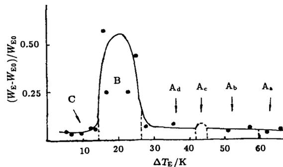
**Fig.2** Experimental result for relative oscillation amplitude under the condition of  $p = 1.5$  MPa,  $q = 200$  kW/m<sup>2</sup>
