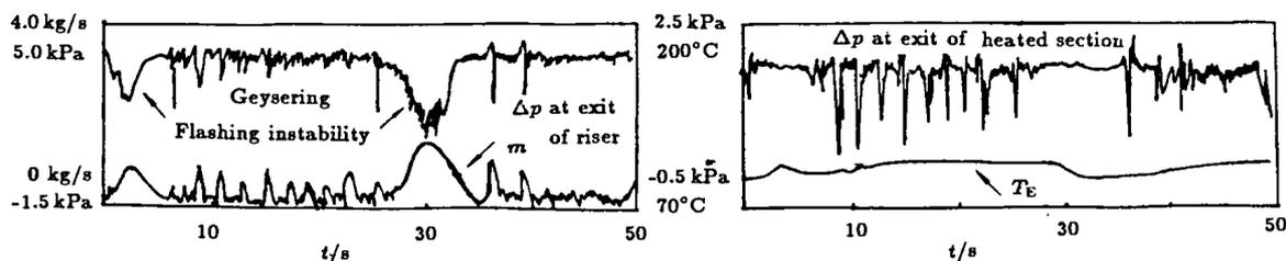
Fig.5 Geysering and flashing instability
