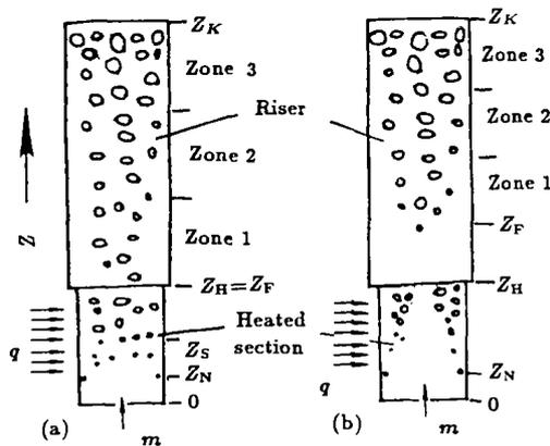
**Fig.1** Two-phase flow pattern in the test loop
