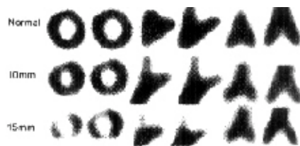
Fig.4 The phantom was moved head 10 and 15 mm along Y -axis compared with normal
