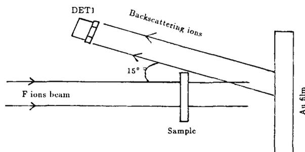
Fig.1 Schematic diagram of the transmission measurement experiment
