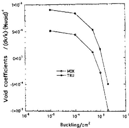
**Fig.7** Void reactivity coefficient variation with buckling
