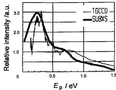
Fig.5 Comparison of transmission grating spectrometer measured X-ray spectrum with that obtained by soft X-ray spectrometer
