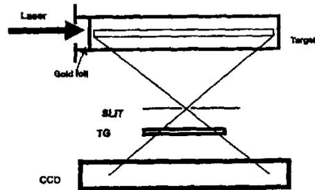
Fig.1 Experimental arrangement to measure the space-resolved X-ray spectra from the inner wall of laser-entered cylindrical gold cavity, which were applied to correct the quantum efficiency of the vacuum oil contaminated X-ray CCD chip
