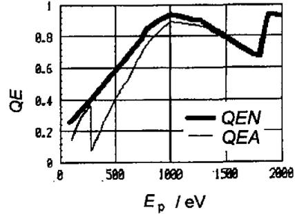
Fig.4 The nominal quantum efficiency of the X-ray CCD in the soft X-ray region, provided by the X-ray CCD manufacturer ( $QEN$ ), and the corrected quantum efficiency of the X-ray CCD ( $QEA$ ) obtained by this work
