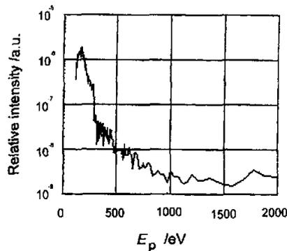
**Fig.3** The typical unfolding X-ray spectrum from the inner wall of the cylindrical cavity end, which is  $800\mu\text{m}$  far from the laser-irradiated gold foil, measured with the transmission grating spectrometer
