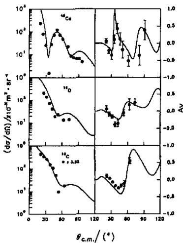
Fig.1 Experimental data of differential cross sections and analyzing powers of 22 MeV polarized proton elastic scattering from  $^{40}\text{Ca}$ ,  $^{16}\text{O}$  and  $^{12}\text{C}$ . Solid lines represent optical-model predictions
