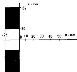
Fig.3 the structure of the  $\phi 124 \times \phi 60 \times 25$  mm magnetic ring
