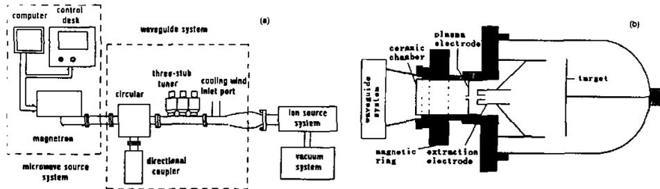
Fig.1 The scheme of the experimental setup of the microwave ion source
