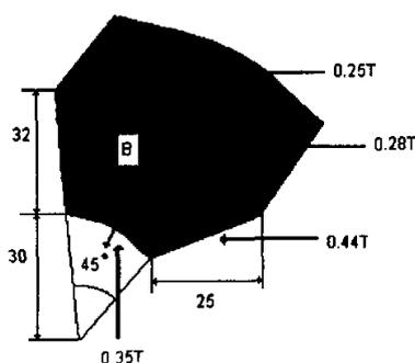
Fig.2 the structure and magnetic field strength of single NdFeB magnetic block
