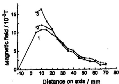
Fig.4 The magnetic field distribution on axis of the  $\phi 124 \times \phi 60 \times 25$  mm magnetic ring. The values of dash dot line are not measured.
