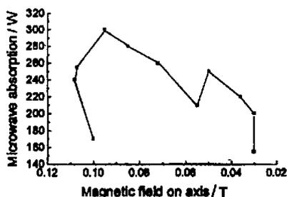
Fig.7 The relation between microwave absorption efficiency and the axial magnetic field
